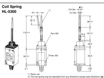
\*3. The operating range of the dog or cam is the top third (i.e. from the tip of the rod) of the whole actuator.
